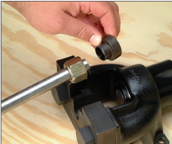
Step 9 Remove the Tube Lift out the tube with preset ferrule and inspect it according to the procedures shown to the right.
