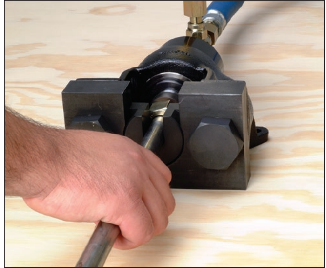
Step 7 Preset the Ferrule Determine the required preset pressure based on the tube size from the table on page 4. Apply hydraulic pressure with a hand or electric pump to advance the piston of the Hyferset. Continue the operation until the predetermined pressure is reached. De-energize the hydraulic power supply or release the valve on the hand pump. The Hyferset piston will retract.
