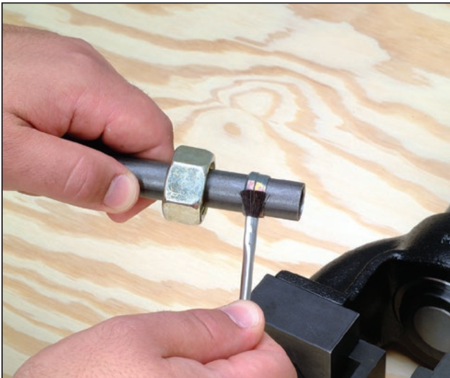
Step 4 Lubricate the Progressive Ring (EO Only) Lubricate the leading outer (bite) edge of the ferrule with lubricant, comparable to the viscosity of STP®. This reduces wear on the die and lowers friction, ensuring that all the force is available to preset the progressive ring.
