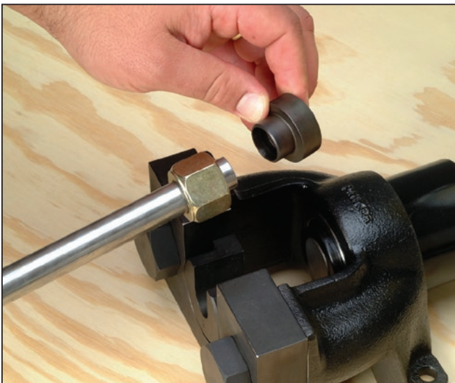
Step 8 Remove the Tube Lift out the tube with preset progressive ring and inspect it according to the procedures shown on the following page.
