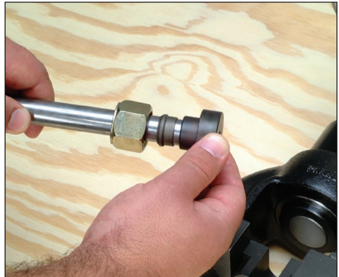
Step 5 Install the Body Die Lubricate the inside of the body die with lubricant (EO only), comparable to the viscosity of STP®. Install the body die over the tube end until the tube bottoms on the die shoulder. Push the nut and progressive ring forward to place the parts in correct position for presetting. The body die will enter the bore of the nut, and the parts will be in the correct position for presetting.
