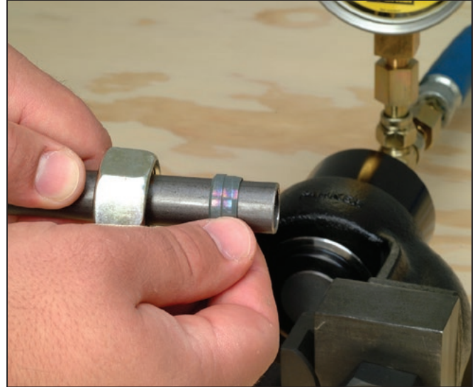
Step 3 Install the Nut and Progressive Ring onto the Tube Slide the nut and progressive ring onto the tube. For EO, the straight pilot section (bite edge) points toward the end of the tube on which it is to be preset, and the raised portion of the progressive ring points toward the nut. For EO-2, slide the functional nut assembly onto the tube with the threaded end of the nut facing the end of the tube to be preset.
